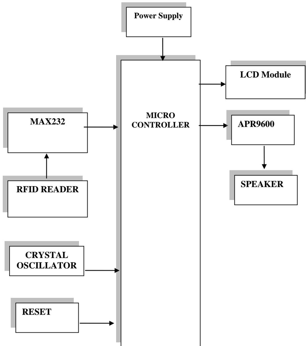
Fig 1: Block Diagram of Proposed System
