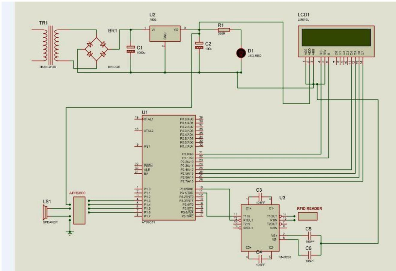
**Fig 7: The Diagram describes all the connections made in the proposed system.**
