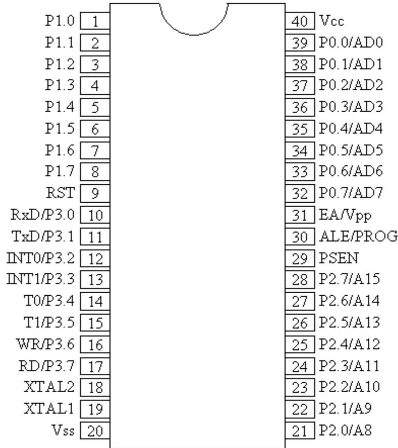
**Fig 2: PIN Diagram of Microcontroller(8052)**
