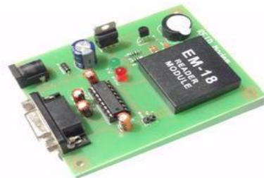
**Fig 4: RFID Reader Module**
