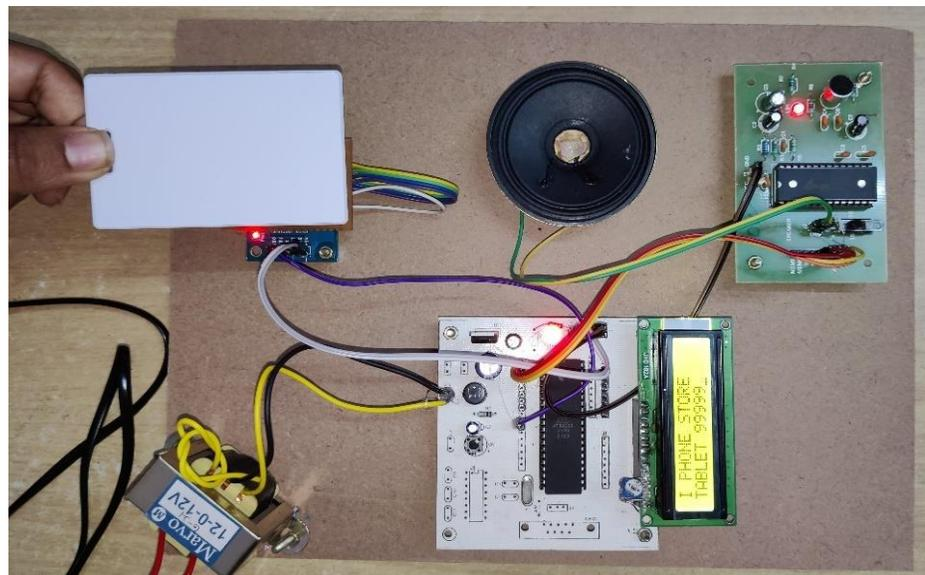
**Fig 9:** The product name and product price will be display and also will be audible at the speaker when there is a contact between RFID Reader and respective Product RFID tag.
