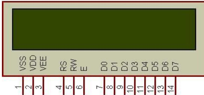
**Fig 3:LCD Display Module**
