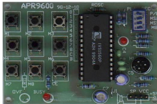
**Fig 6: APR9600 Experimental Board**
