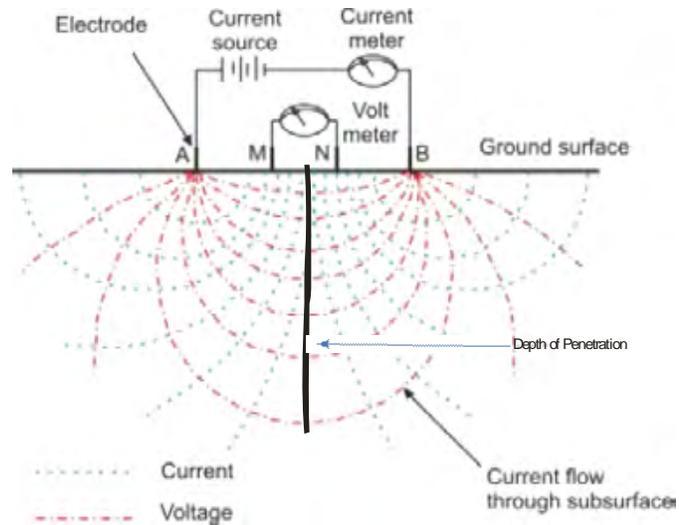
Fig 5. Current flow in the ground for resistivity determination
