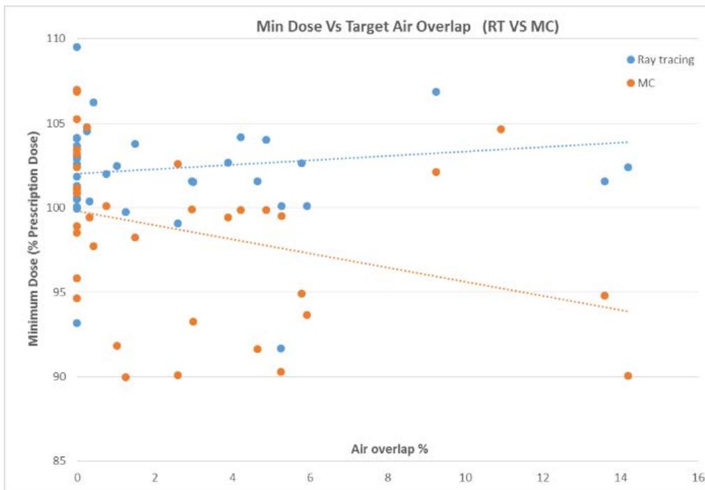
Fig. 4 Min Dose with Increasing Target Air Overlap - Ray Tracing vs Monte Carlo
