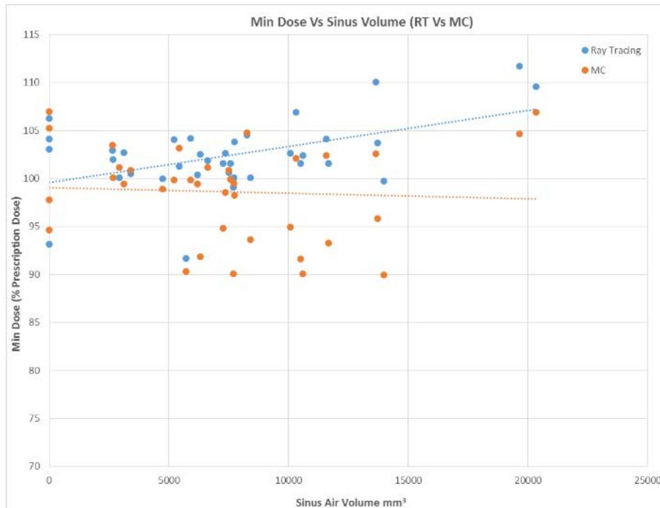
Fig. 6 Min Dose with increasing adjacent Sinus Air Volume - Ray Tracing vs Monte Carlo
