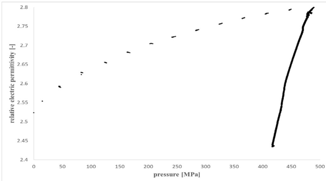
Figure 7. Diagram of relative electric permittivity vs. pressure during and after compression.
