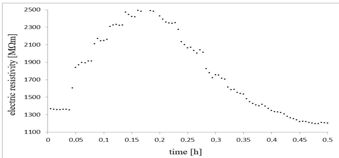
Figure 8. Diagram of electric resistivity vs. time during compression.
