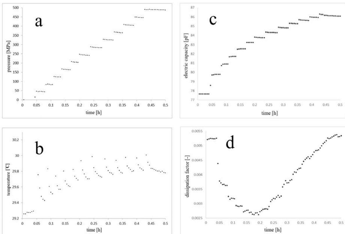
Figure 3. Quantities measured directly vs. time, a – pressure, b – temperature, c – capacitance, d – dissipation factor.
