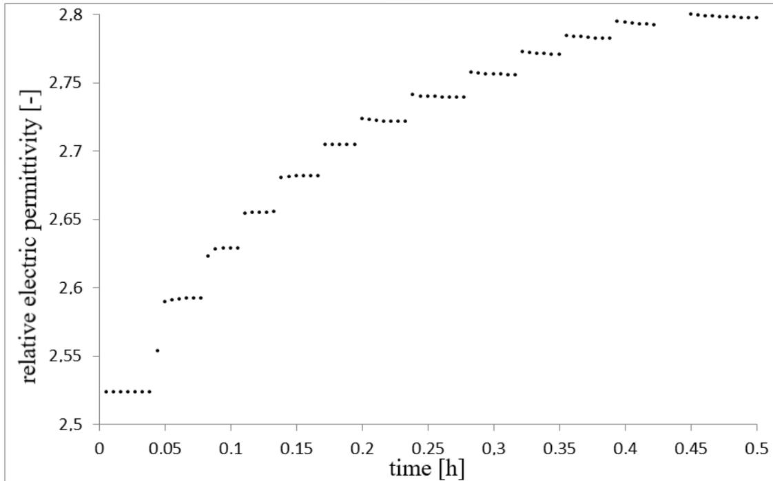
Figure 5. . Diagram of relative electric permittivity vs. time diagram during compression.
