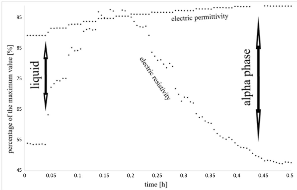
Figure 11. Comparison of the dependence of electric permittivity and electric resistivity on time during compression.
