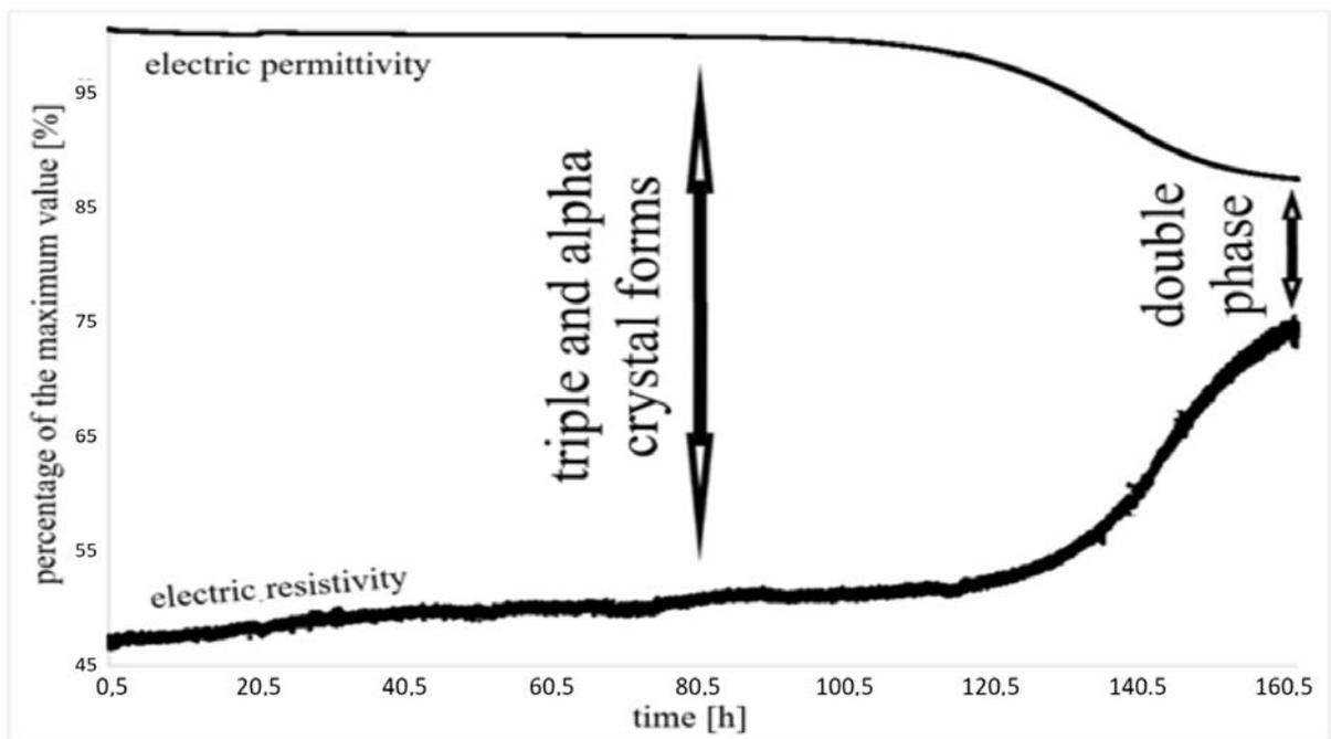
Figure 12. Comparison of the dependence of electric permittivity and electric resistivity on time after compression.
