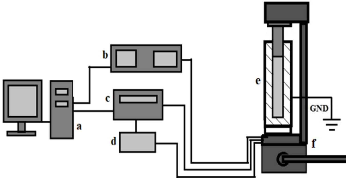
Figure 2. Data acquisition system: a – Computer with LabVIEW based acquisition system, b – RLC automatic bridge, c – multi-meter with multiplexer, d – temperature reference system, e – high pressure chamber, f – hydraulic press.
