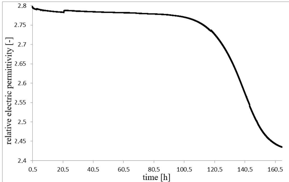
Figure 6. Diagram of relative electric permittivity vs. time after compression.
