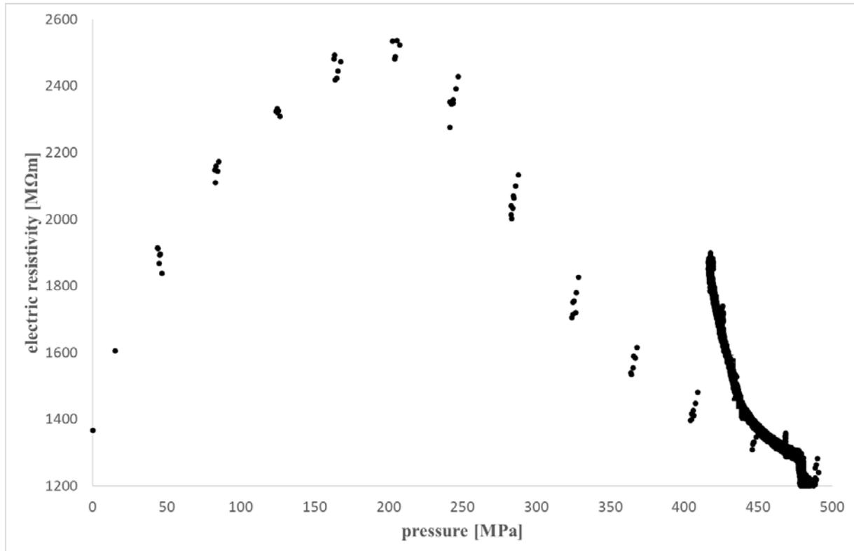
Figure 10. Diagram of electric resistivity vs. pressure during and after compression.
