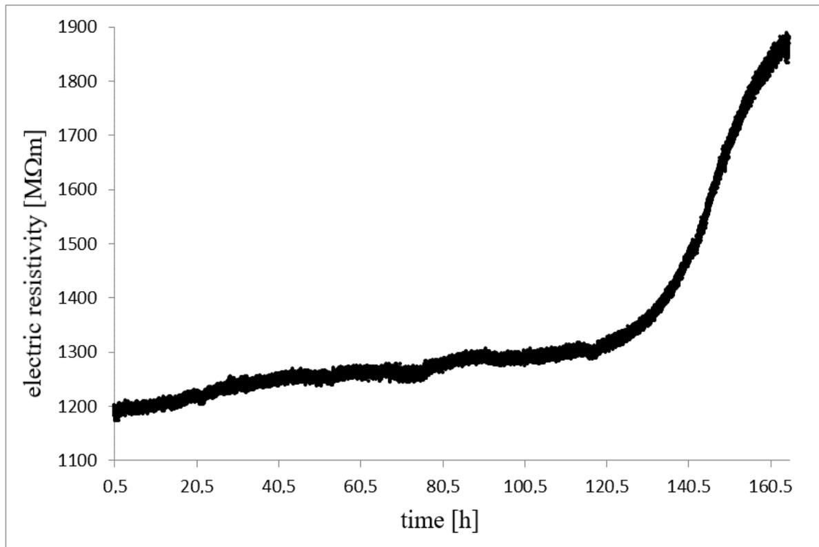
Figure 9. Diagram of electric resistivity vs. time after compression.
