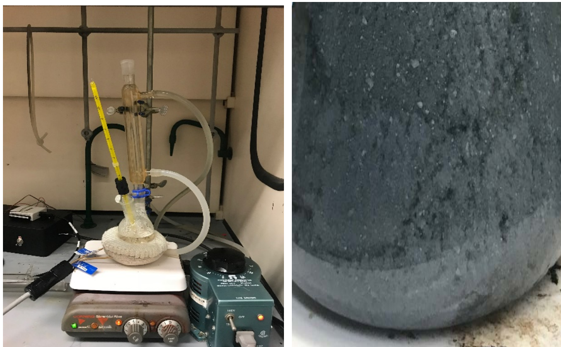
Figure 1. (a) Solution was refluxed for a period of three hours and (b) grey-green colored precipitate on the bottom.
