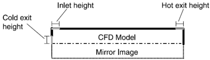
Figure 6: Schematic of the CFD model, shown with mirror image [14].
