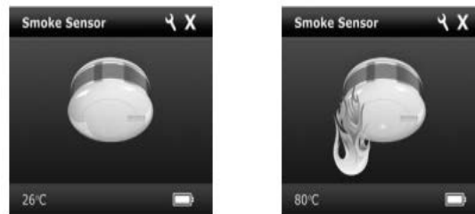
Fig. 3 Fibaro Fire detection status
