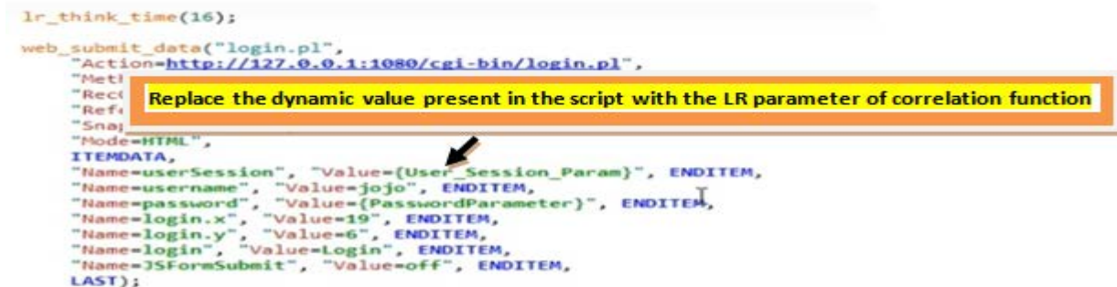
Fig 11: Replace the dynamic value present in the script with the LR parameter of correlation function
