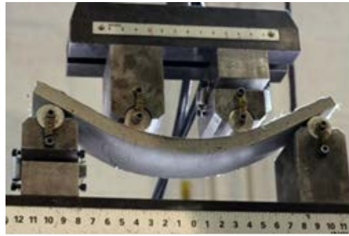
Fig 13: Concrete under force, small and narrow cracks happen instead of one big crack
