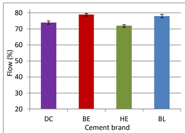
**Figure 3:** Effect of cement brands on flow of mortar mixes (Error bars equal average  $\pm$  standard deviation)
