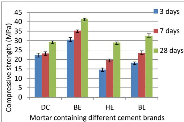
**Figure 4:** Variation of Compressive strength with age (Error bars equal average  $\pm$  standard deviation)
