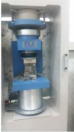
**Figure 2:** ADR-Auto compression testing machine
