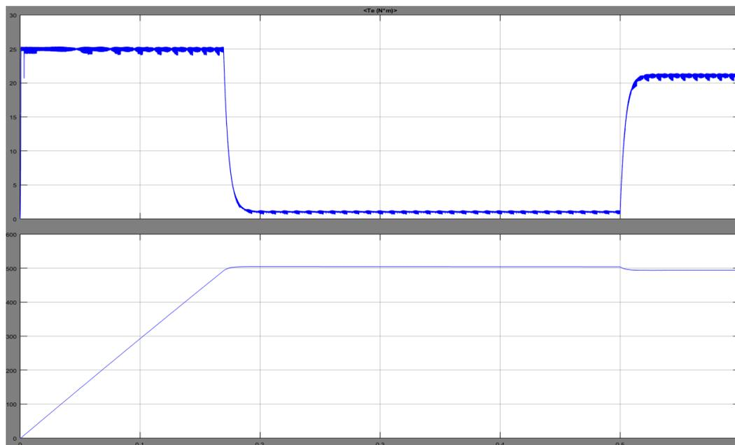
Fig. 10(b) Total torque and speed response for speed reference equal to 500 RPM and load torque of 20N.m applied at  $t=5$ sec
