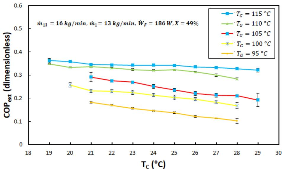
Fig. 11  $COP_{ext}$  against  $T_C$  for different  $T_G$  at  $X = 49\%$ .
