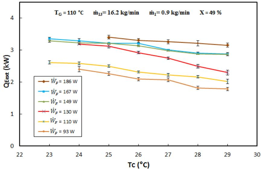
Fig. 13  $\dot{Q}_{Ext}$  against  $T_C$  for different  $\dot{W}_F$ .
