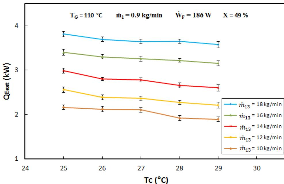
Fig. 15  $\dot{Q}_{Ext}$  against  $T_C$  for different heat water mass flow rates.
