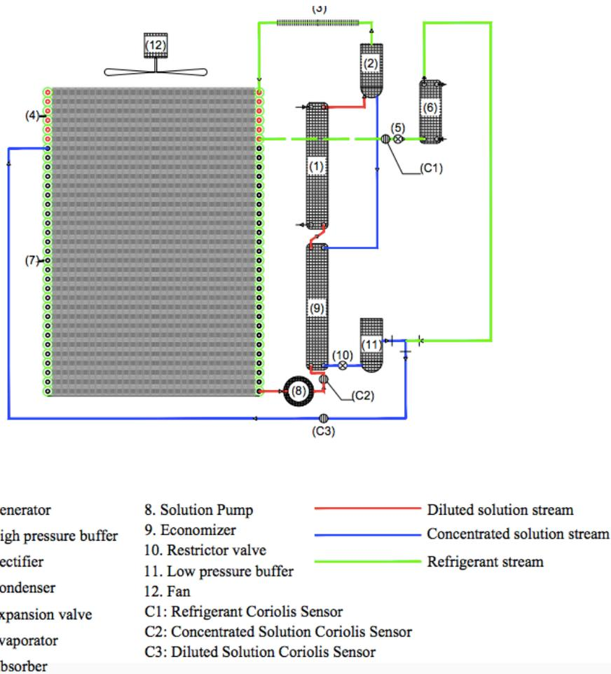
Figure 1. Schematic diagram of the system.
