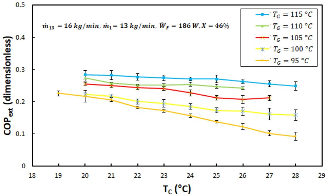
Fig. 8 COP<sub>ext</sub> against T<sub>C</sub> for different T<sub>G</sub> at X = 46%.
