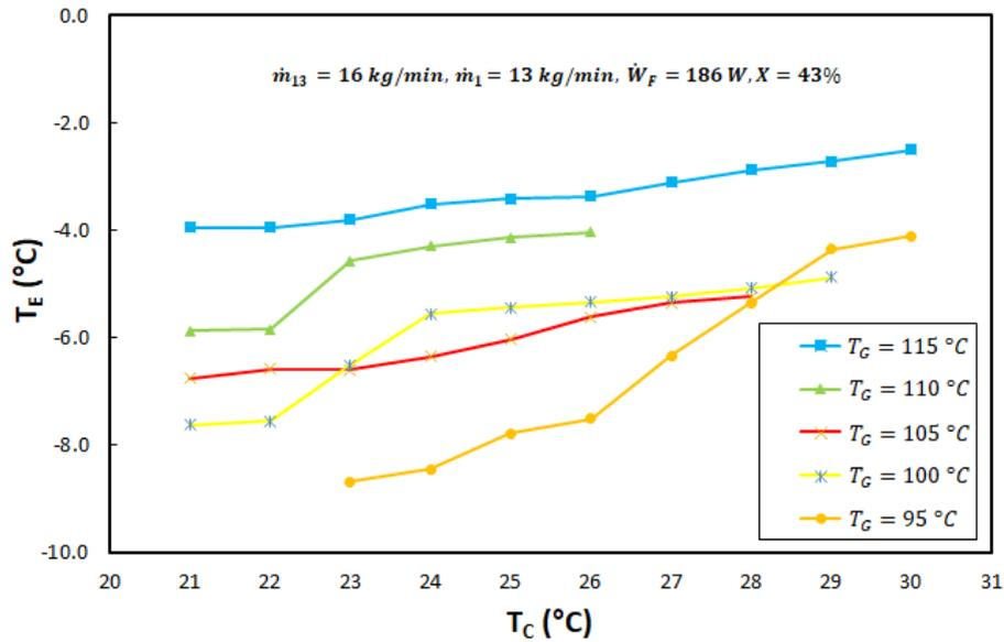
Fig. 6 Evaporator temperature against T<sub>C</sub> for different T<sub>G</sub> at X = 43%.
