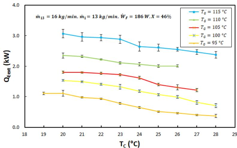
Fig. 7  $\dot{Q}_{Eext}$  against T<sub>C</sub> for different T<sub>G</sub> at X = 46%.
