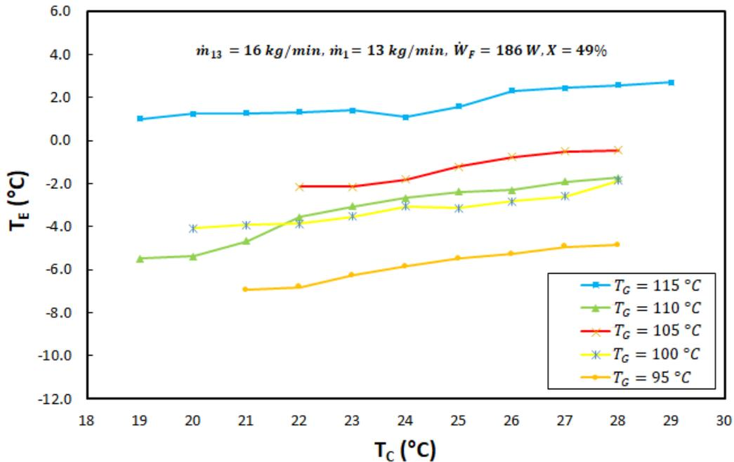
Fig. 12 Evaporator temperature against  $T_C$  for different  $T_G$  at  $X = 49\%$ .
