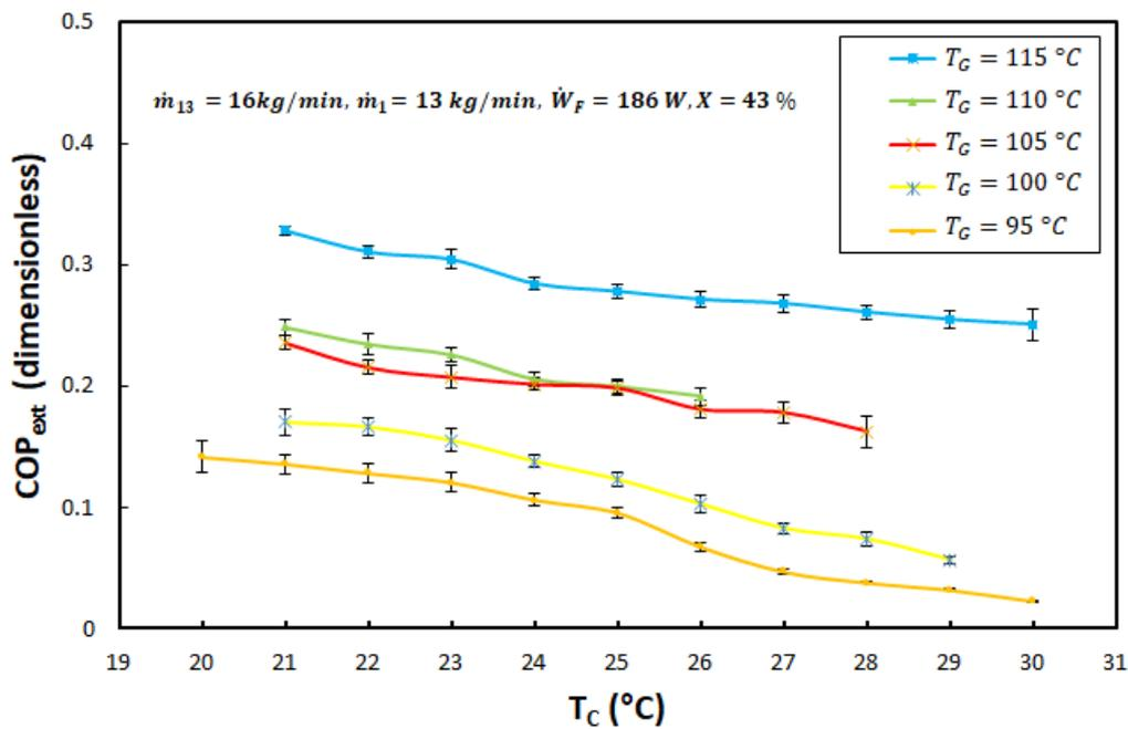
Fig. 5 COP<sub>ext</sub> against T<sub>C</sub> for different T<sub>G</sub> at X = 43%.
