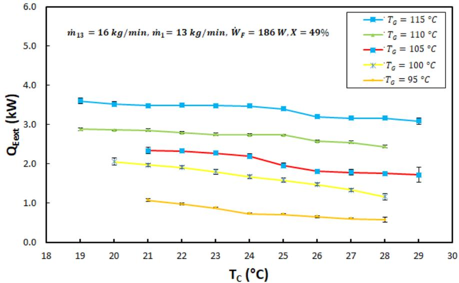
Fig. 10  $\dot{Q}_{Ext}$  against  $T_C$  for different  $T_G$  at  $X = 49\%$ .
