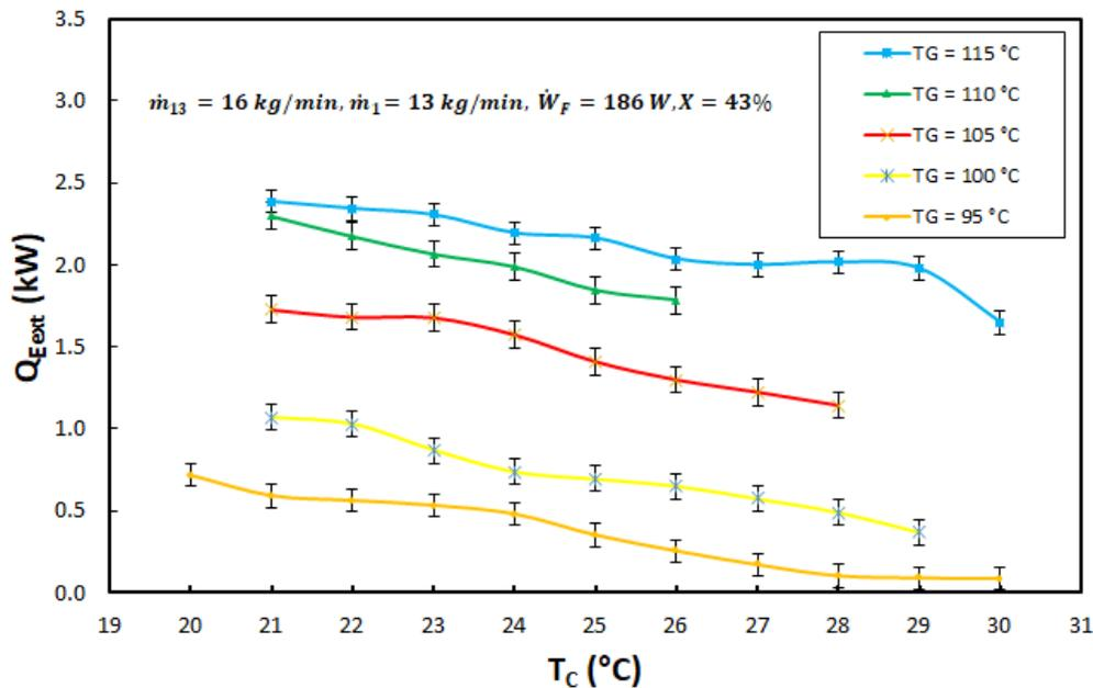
Fig. 4  $\dot{Q}_{Ext}$  against  $T_C$  for different  $T_G$  at  $X = 43\%$ .
