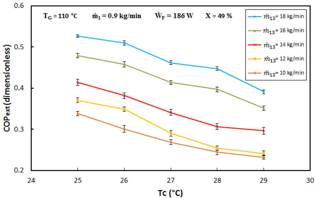
Fig. 16  $COP_{ext}$  against  $T_C$  for different hot water mass flow rates.
