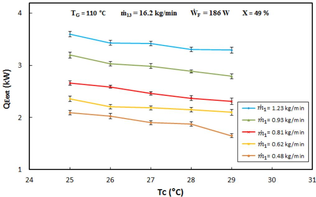
Fig. 17  $\dot{Q}_{Ext}$  against  $T_C$  for different solution mass flow rates.
