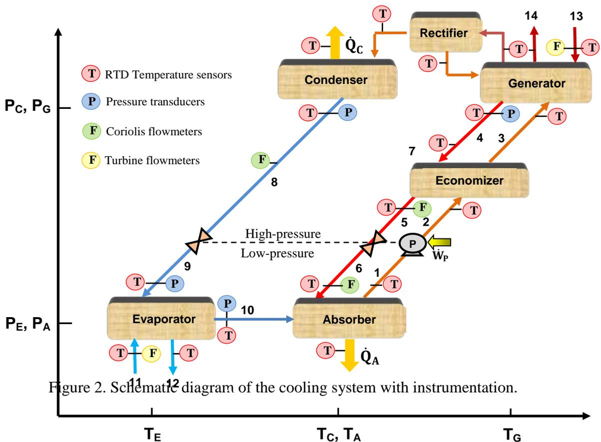
Figure 2. Schematic diagram of the cooling system with instrumentation.
