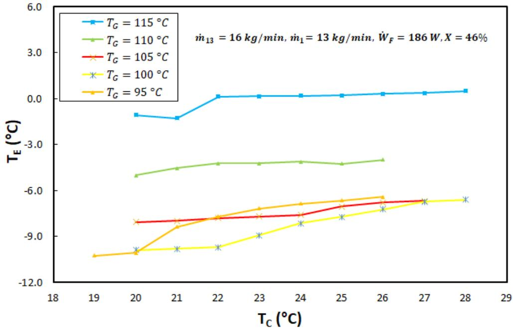
Fig. 9 Evaporator temperature against  $T_C$  for different  $T_G$  at  $X = 46\%$ .
