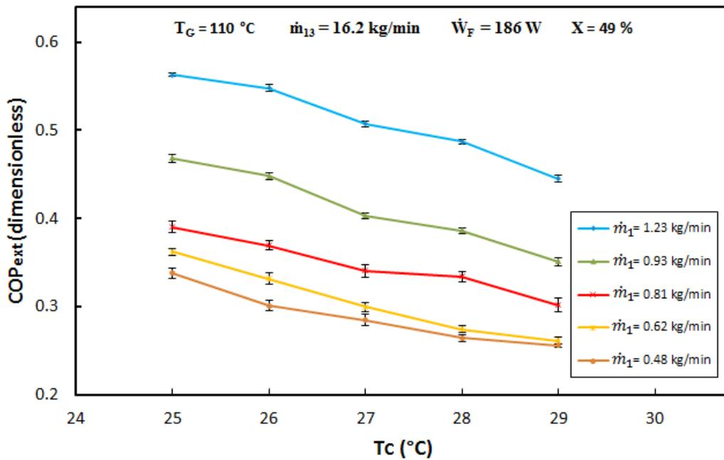
Fig. 18 COP<sub>ext</sub> against T<sub>c</sub> for different solution mass flow rates.
