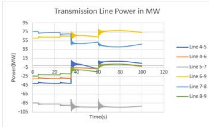
Figure 3: Power flow in the transmission line
