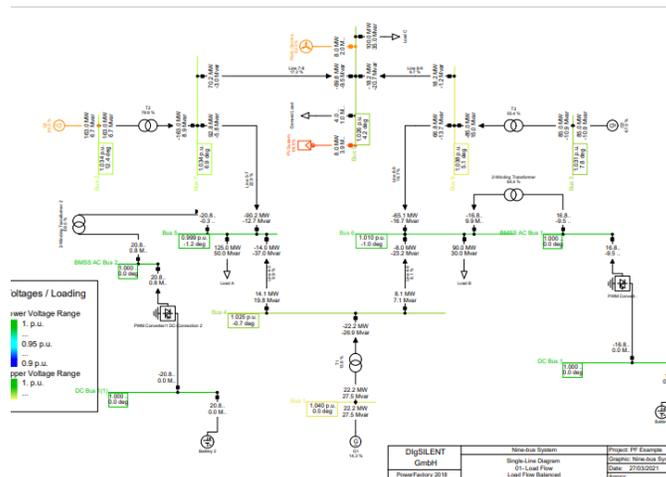
Figure 1: Modified IEEE 9 bus system model
