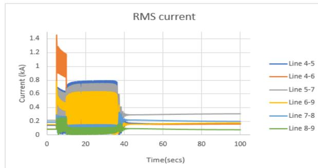
Figure 6: Transient line current under 5secs fault
