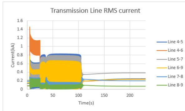
Figure 7: Transient line current under 20secs fault
