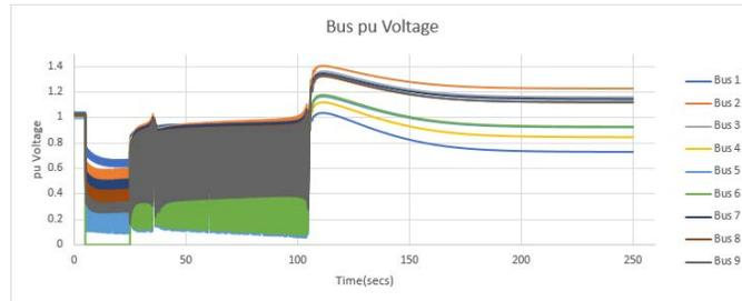
Figure 5: Bus Bar RMS voltage under a symmetrical fault
