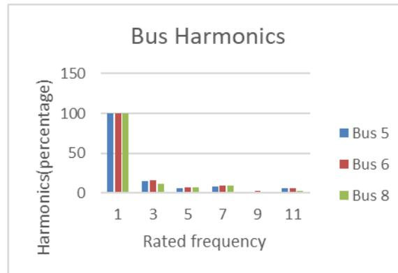
Figure 18: System harmonics with DG and BESS
