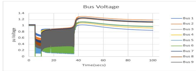
Figure 4: Bus Bar RMS voltage under a symmetrical fault
