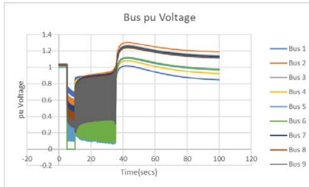
Figure 8: Bus per-unit (pu) voltage with wind turbine connected
