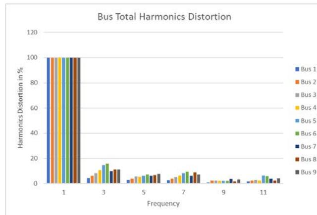
Figure 16: System harmonic distortion with DG and BESS connected
