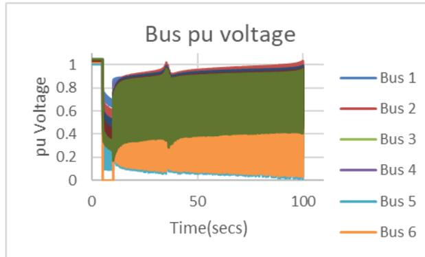
Figure 9: Bus pu voltage with PV connected
