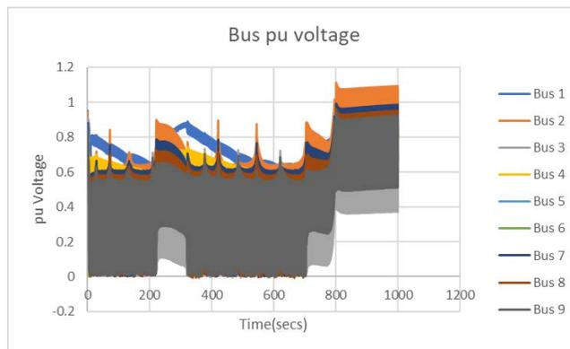
Figure 12: System behaviour under symmetrical fault after 1000s
