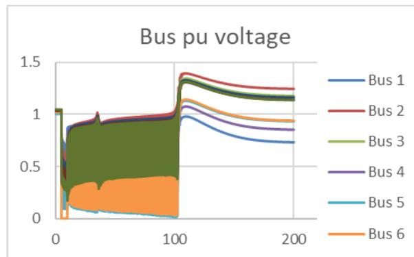
Figure 10: Bus pu voltage with PV connected after 200s
