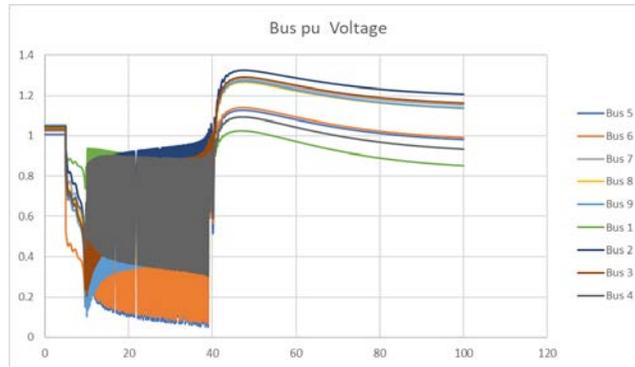
Figure 13: System (without BESS) behaviour under asymmetrical fault
