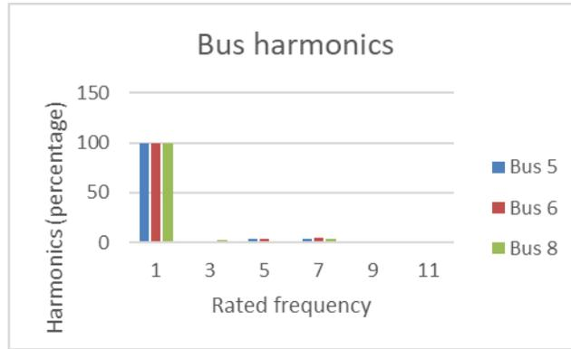
Figure 17: System harmonics without DG and BESS
