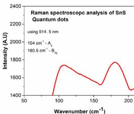
Figure 6. Raman spectra of SnS quantum dots
