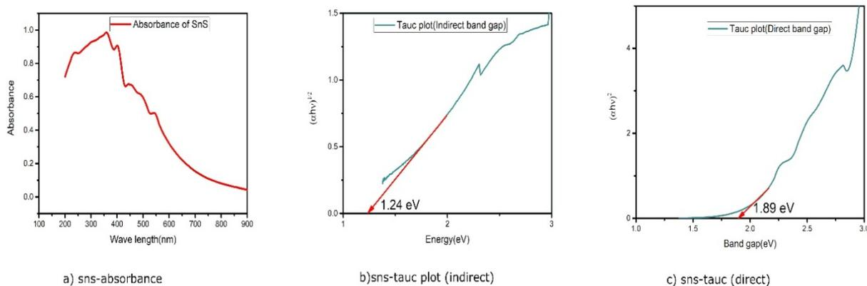
Figure 5. (a) Absorption spectrum of SnS nanoparticles. (b) Tauc plot for indirect band gap. (c) Tauc plot for direct band gap
