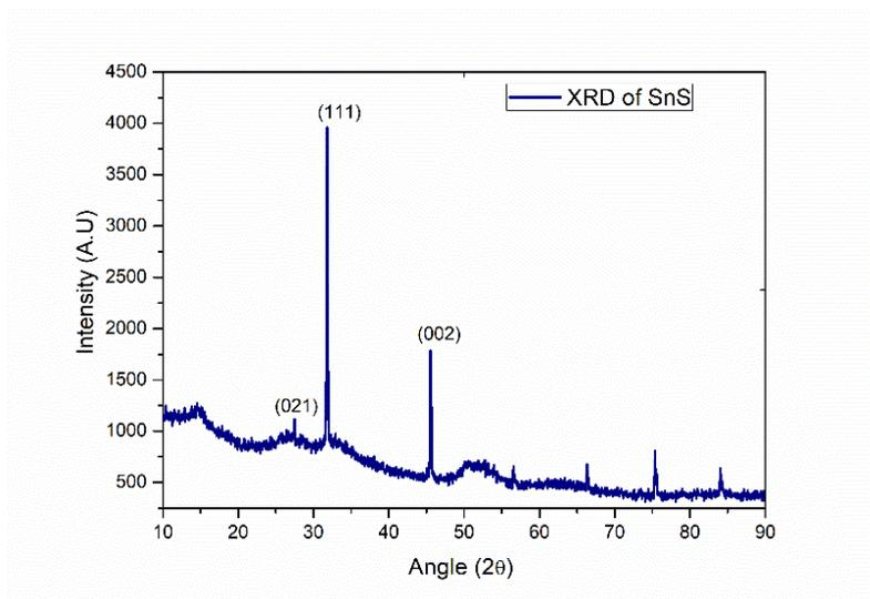
Figure 2. XRD pattern of synthesized SnS nanoparticles
