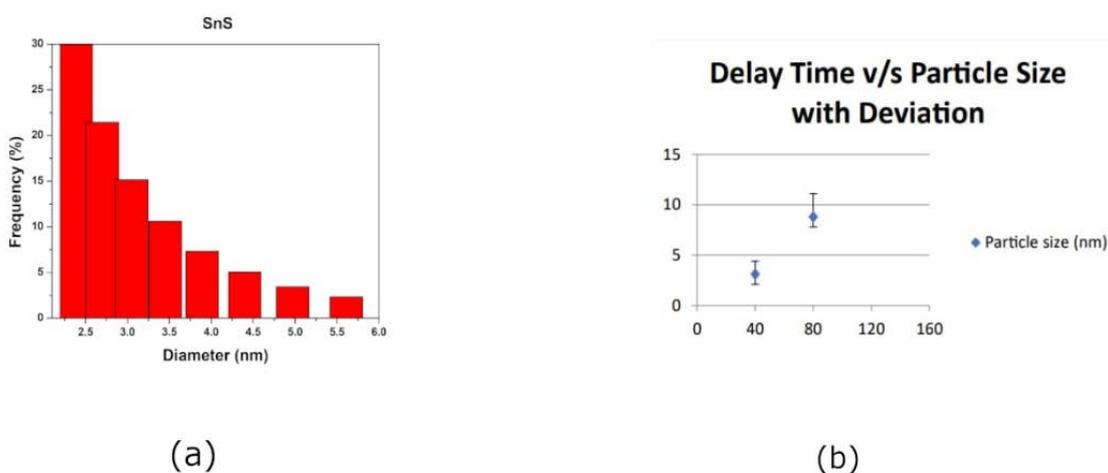
Figure 1(a). Histogram showing the size distribution of SnS nanoparticles. (b) Graph showing variation b/t Delay time and SD with Particle size
