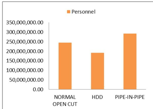
Fig 5 Cost Comparison for Personnel Using Normal Open Cut, HDD and Pipe-In-Pipe for a 20” x 15km Pipeline
