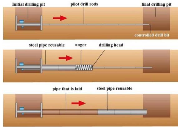
Figure 2 Steps in HDD Pipe Lay
