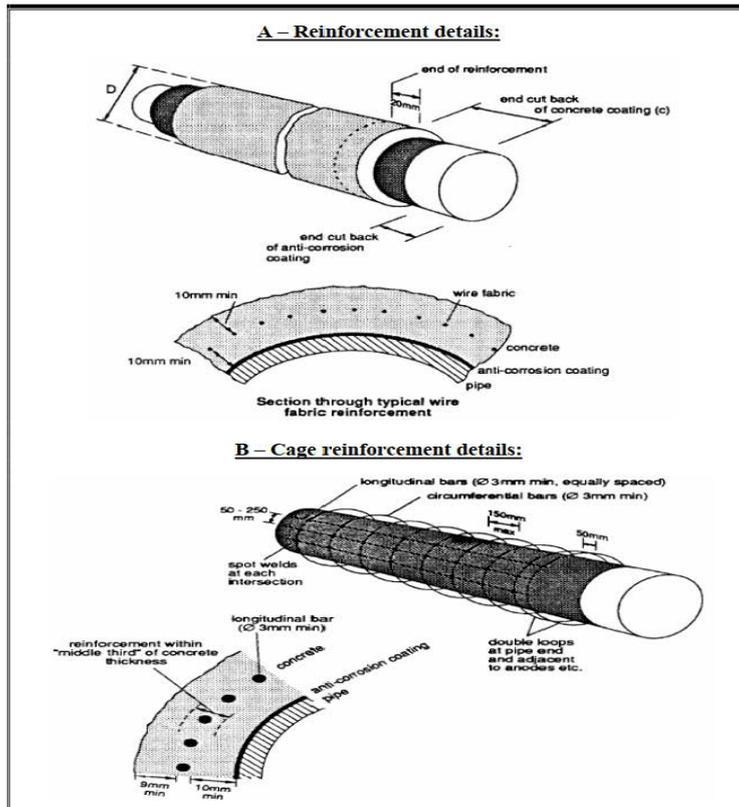
Fig 4 Concrete Coating of Pipe outer surface
