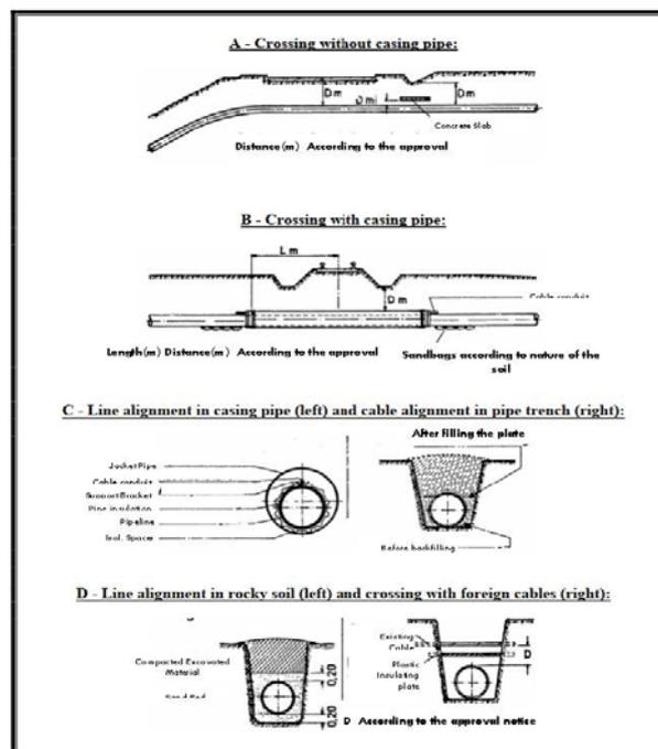
Fig 3 Pipe-in-pipe Profiles and Line Allignment
