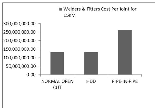
Fig 7 Cost Comparison for WELDERS & FITTERS Cost Per Joint for 15KM Using Normal Open Cut, HDD and Pipe-In-Pipe for a 20” x 15km Pipeline
