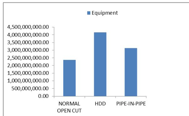
Fig 6 Cost Comparison for Equipment’s Using Normal Open Cut, HDD And Pipe-In-Pipe for a 20” x 15km Pipeline
