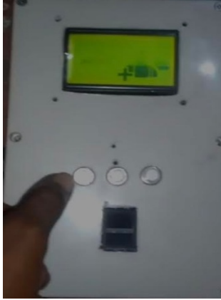
Fig 2: Internet of Things (IoT) Biometric voting system
