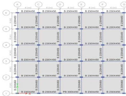
Fig. 3.2: Plan view of RC building without infill considering wall load
