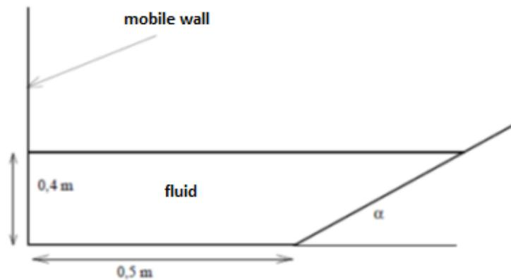
Figure 5: Domain used for simulating the impact of waves.
