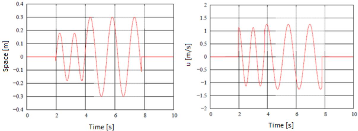
Figure 6: Displacement (up) and speed (down) of the wave generator on the horizontal axis.
