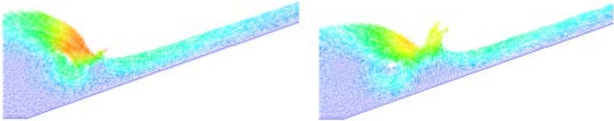
Figure 8: Flow velocity vector in time 2.71 s (left) and 2.81 s (right).
