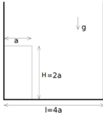
Figure 1: Geometry used in the dam break simulation.
