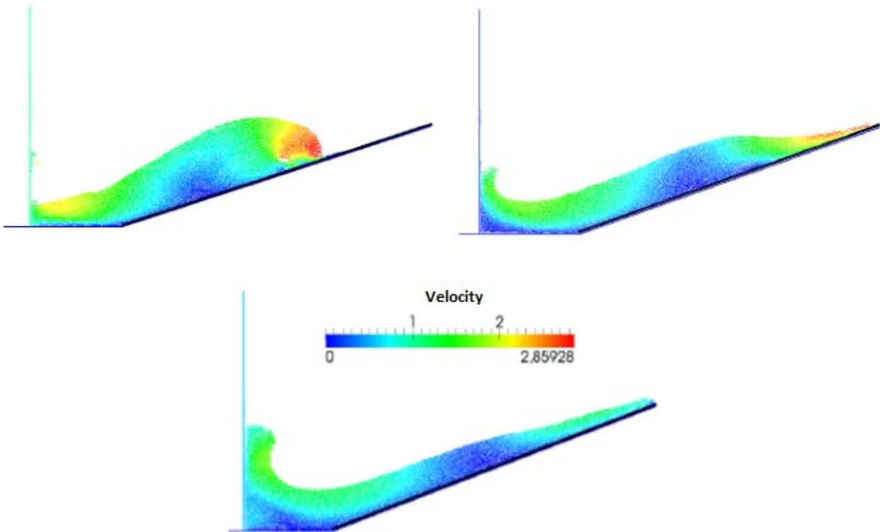
Figure 7: Flow development in 2.12 s (top left), 2.23 s (top right) and 2.38 s (down).
