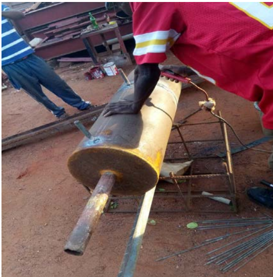
Figure 6: The chimney and the boiler unit
