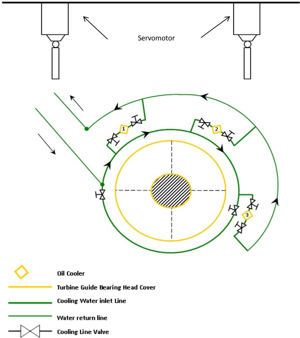
Figure 4: Cooling System with Three (3) Oil Coolers
