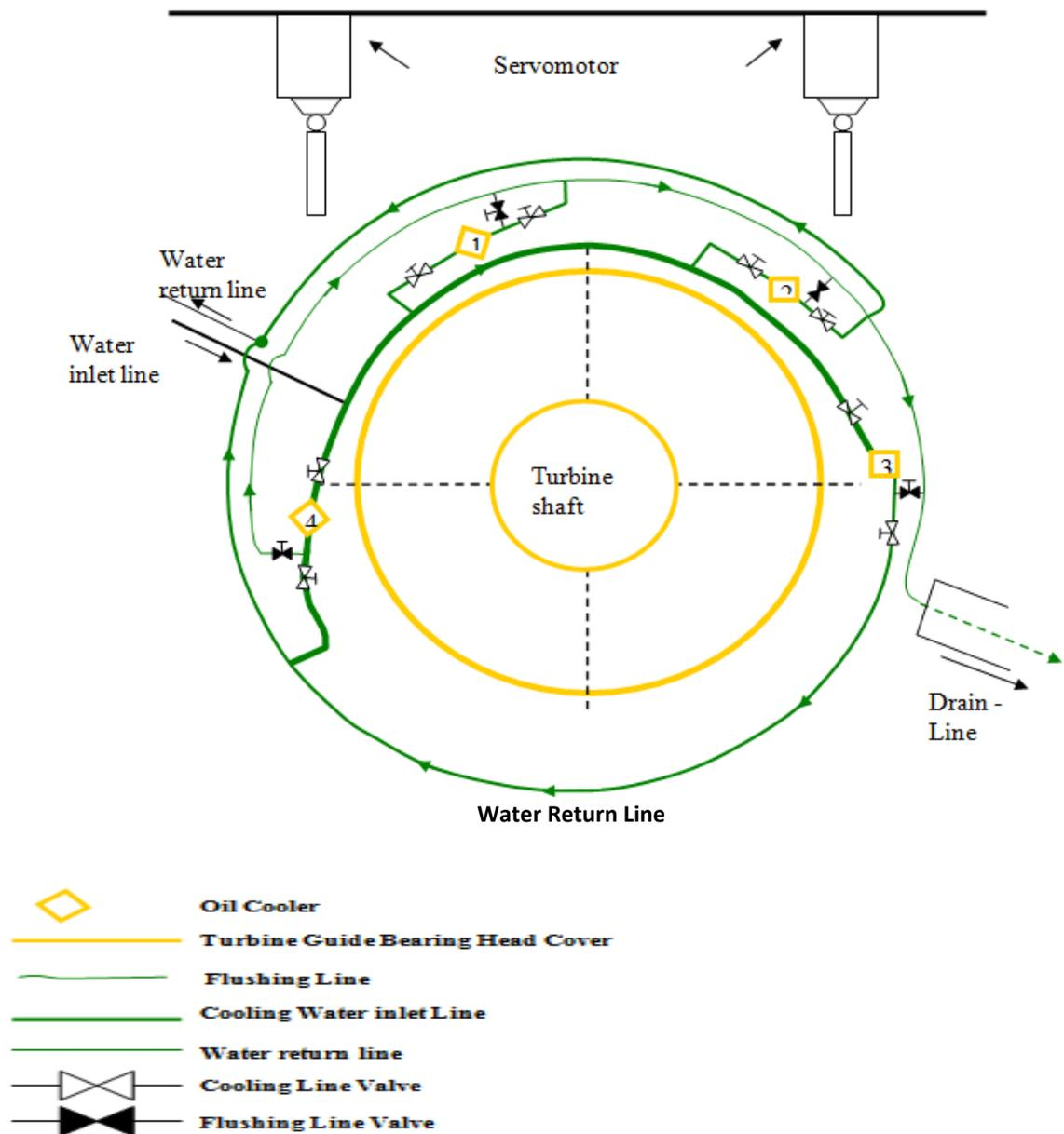
Figure 5: Cooling System with Four (4) Oil Coolers
