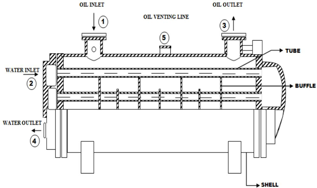
Figure 1: Block Diagram of Oil Cooler
