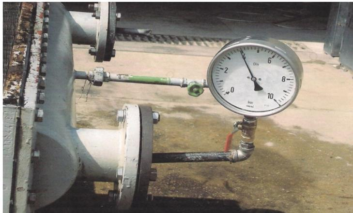
**Figure 3: Radiator Pressure Test Experimental Setup (at Shiroro Power Station)**
