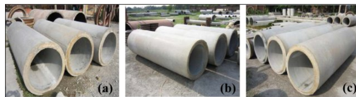
Fig. 5 Construction pipes: (a) Pipes without jute fiber reinforcement, (b) pipes with untreated jute fiber reinforcement, (c) pipes with chemically modified jute fiber reinforcement (27)
