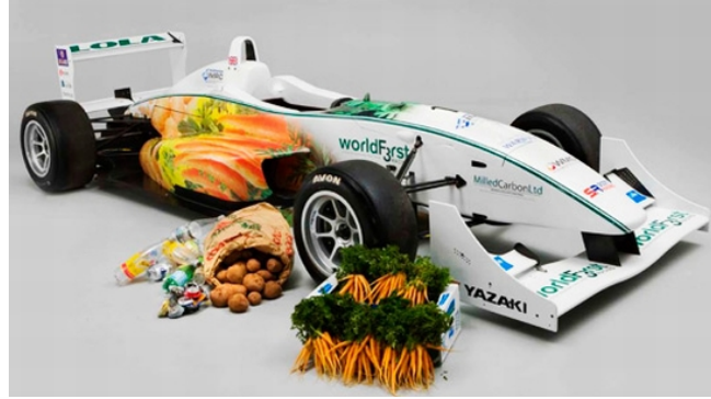
Fig. 2. Formula 3 racing car built from renewable materials powered by waste derivative fuel.
