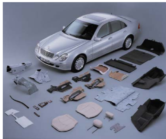
Fig. 3 Biocomposite body panels and components of E-class Mercedes (28)
