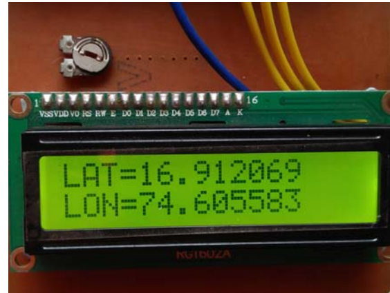
Fig(6):GPS + LCD showing lat & long information
