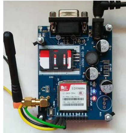
Fig(4): GSM interface with Arduino
