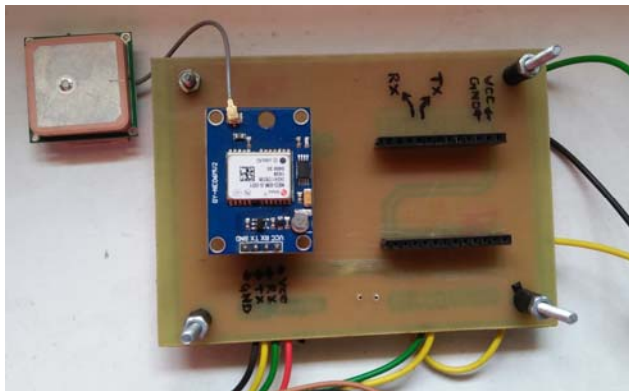
Fig(3):GPS interface with Arduino
