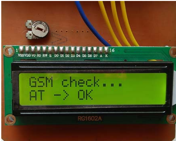
Fig(5): LCD interface with Arduino
