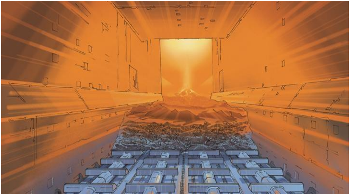
Fig 2.1: The Inner View of a Grate Cooler with Clinker Nodules on the Grate Plate. Source: (Ahamed et al. , 2012)
