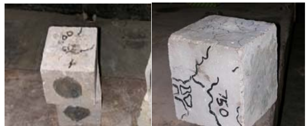
Fig: 5.2 Surface cracking
