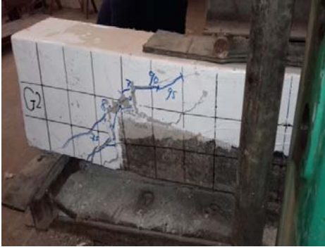
Photo1. Girder G2 - Strengthening Length = 2L/3
