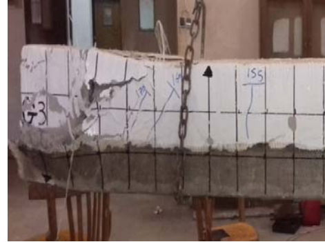
Photo2. Girder G3 - Strengthening Length = L
