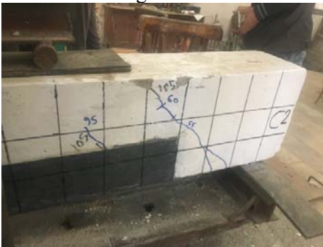
Photo3. Girder C2 - Strengthening Length = 2L/3 .
