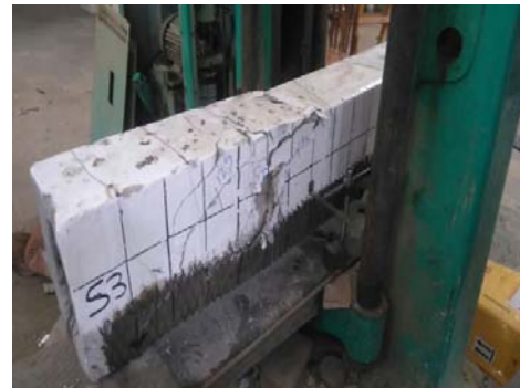
Photo6. Girder S3 - Lateral, Bottom Strengthening Length = L
