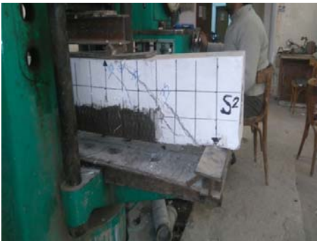
Photo5. Girder S2 - Lateral, Bottom Strengthening Length = 2L/3
