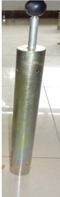
Fig. 3: Hammer of modified proctor.
