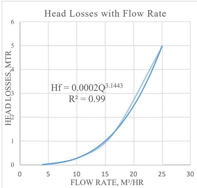
Figure # 3: Head losses vs Flow Rate
