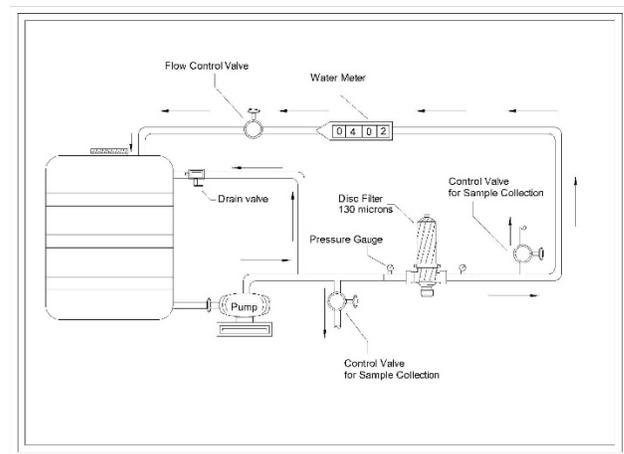
Figure # 1: Layout plan of Experimental Plan.
