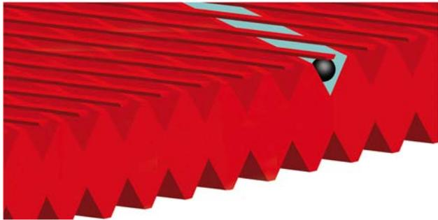
Figure # 2: Groove pattern of Disc Filter
