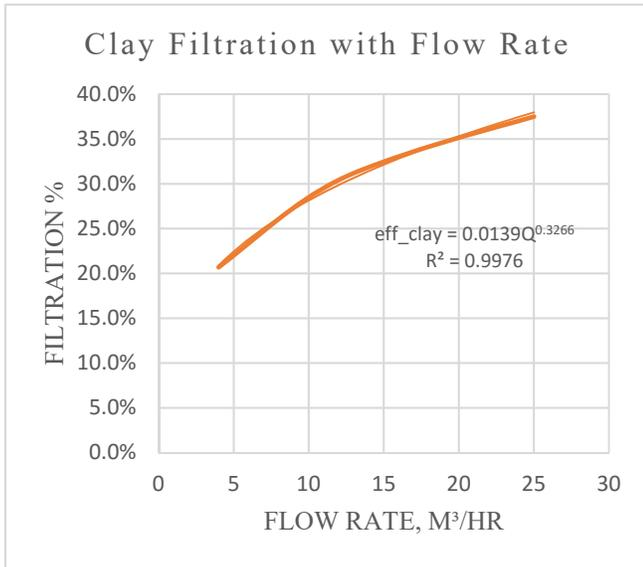
Figure # 5: Percentage of Clay filtered vs Flow Rate.
