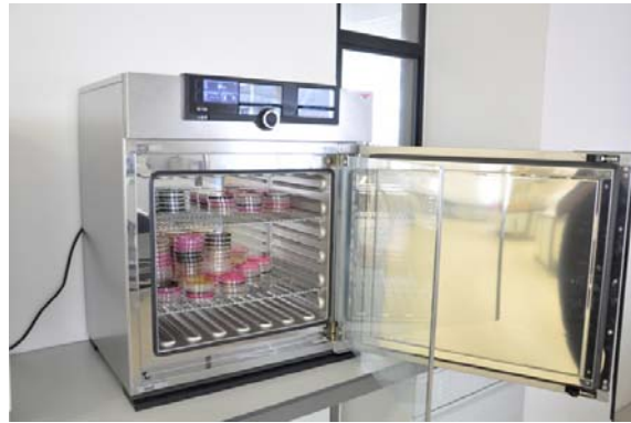
Fig. 2 Images of Agar Plate placed in an Incubator Machine at 37°C
