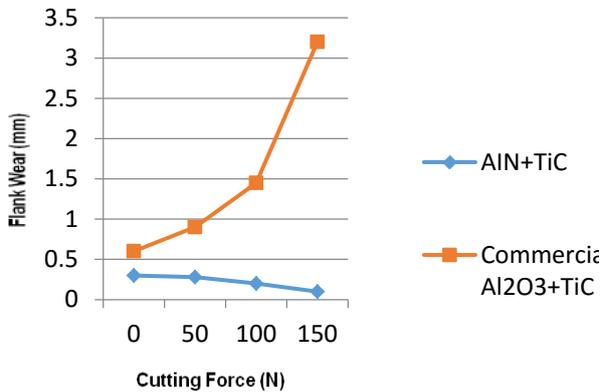
**Fig. 5 Cutting Force Vs Flank wear**
