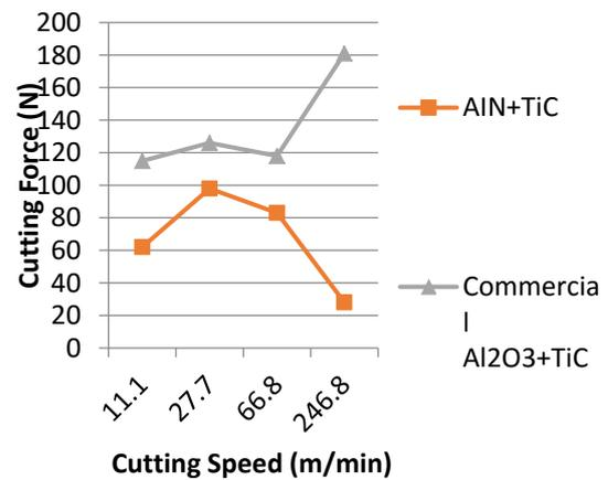
Fig. 2 Cutting Speed Vs Cutting Force
