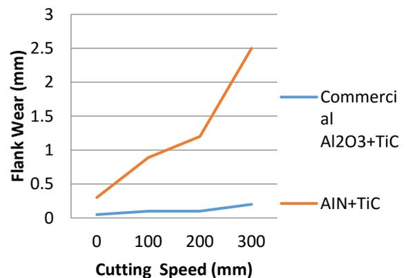
Fig.3 Cutting Speed Vs Flank Wear
