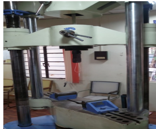
Fig4.3 Universal testing machine (UTM)
