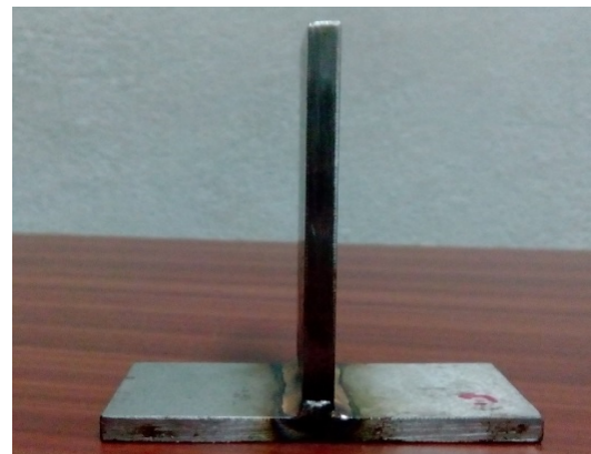
Fig 4.1 welded T-joint material by Tungsten Inert Gas welding process
