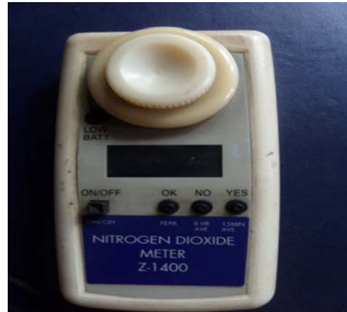
Plate 3: NO 2 meter Z – 1400 for Nitrogen dioxide monitoring
