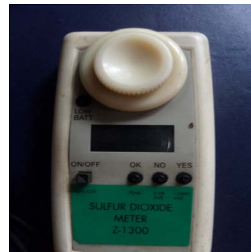
Plate 4: SO 2 meter Z – 1300 for Sulphur dioxide monitoring
