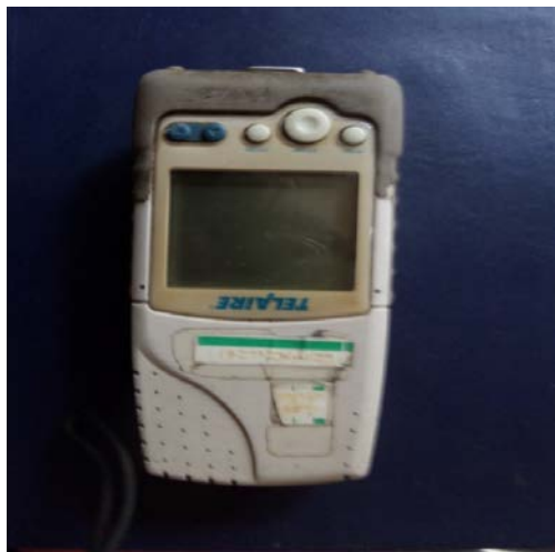
Plate 2: Telaire 7001 CO 2 and Temperature monitor
