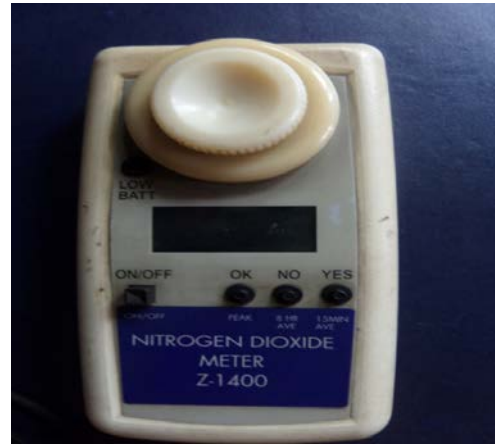
Plate 3: NO 2 meter Z – 1400 for Nitrogen dioxide monitoring
