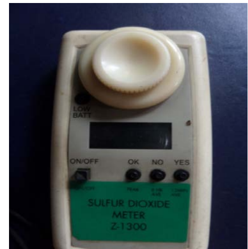
Plate 4: SO 2 meter Z – 1300 for Sulphur dioxide monitoring
