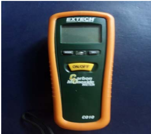
Plate 1: Extech CO10 meter for Carbon monoxide monitoring
