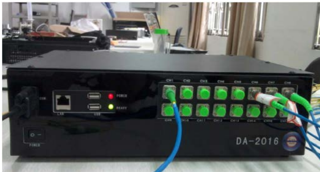
Fig. 11 Integrated optical fiber grating demodulation system.
