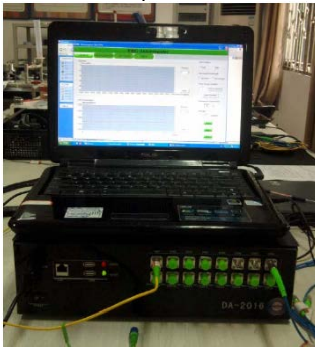
Fig. 11 Integrated optical fiber grating demodulation system.
