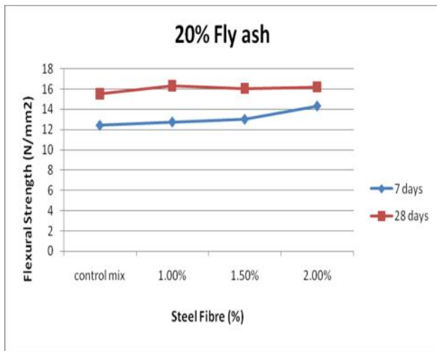
Figure 3: Flexural Strength of SFRC(20% Flyash) & Control Mix
