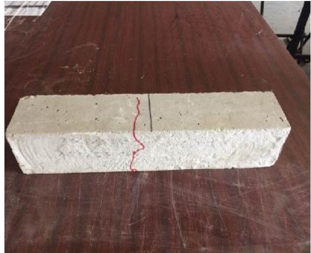
Fig: 2 Testing of Flexural Strength of Beam (Specimen after test)
