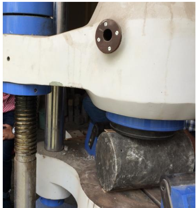
Fig 8: Specimen before Split Tensile Strength Test
