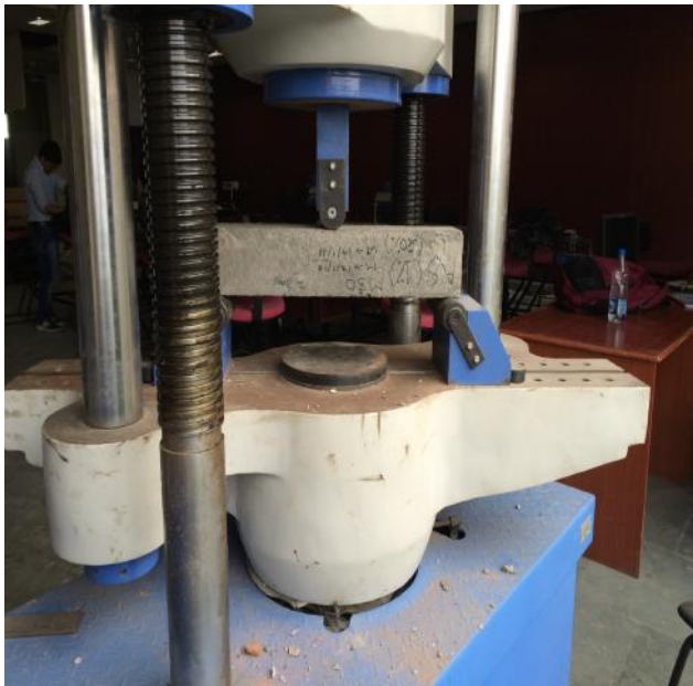
Fig: 1 Testing of Flexural Strength of Beam (Specimen before test)
