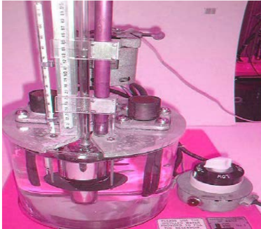
Fig (1): laboratory apparatus Measurement of Specific Heat Capacity
