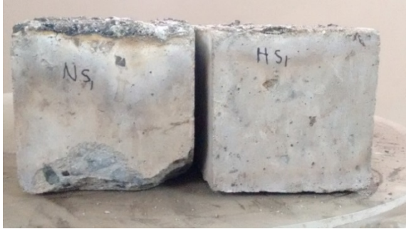
Fig. 6 Effect of Fire on Concrete
