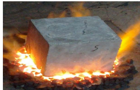
Fig.5 Concrete Exposed to Fire
