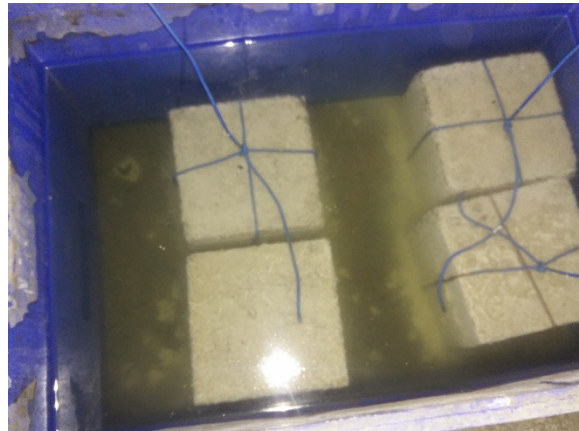
Fig.4 Concrete Exposed to Acid
