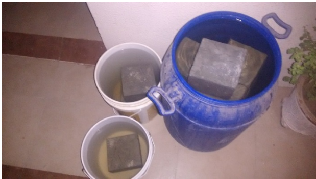
Fig.6 Concrete Exposed to Sea water
