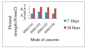
Fig. 8 Flexural strength Chart
