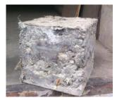
Fig.7 Specimen Before and After Sulphate Attack
