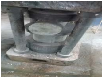
Fig 5. Specimen under Split Tensile Test
