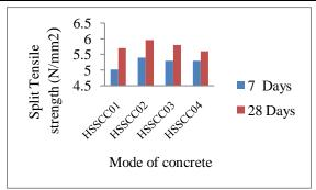
Fig 6: Split Tensile strength Chart
