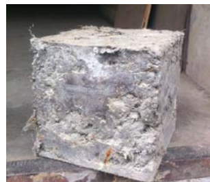
Fig.7 Specimen Before and After Sulphate Attack
