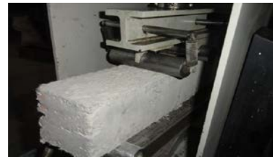
Fig. 7 Specimen Under Split Tensile Test
