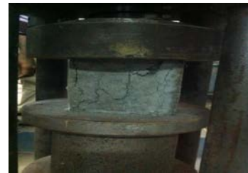
Fig. 3 Cube Under Compression Test
