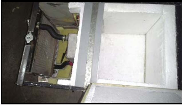
Fig. 6.2 TEC assembled to cooling cabin
