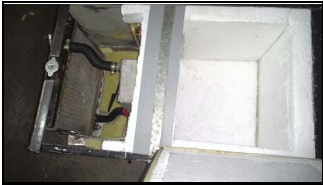
Fig. 6.2 TEC assembled to cooling cabin
