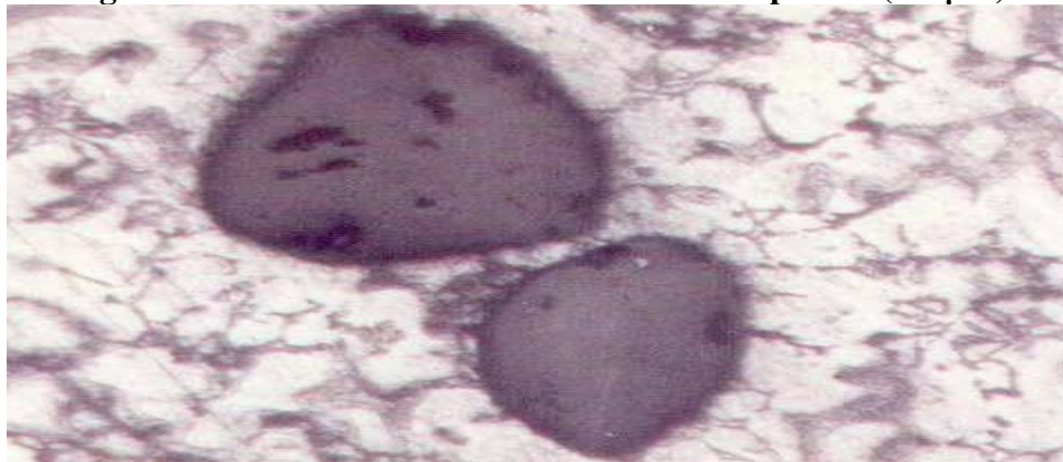
Fig.7 Microstructure of AA7075/ 6% SiC composites (Higher magnification)
