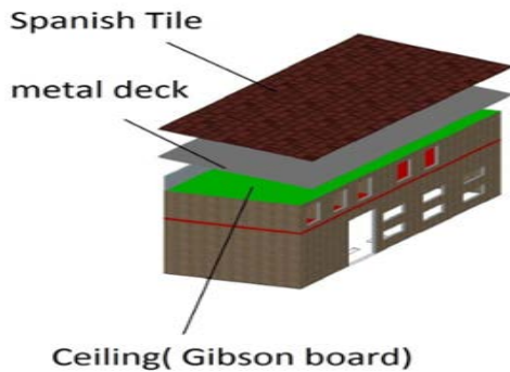
Fig 6 The roof of the factory building without the insulating material
