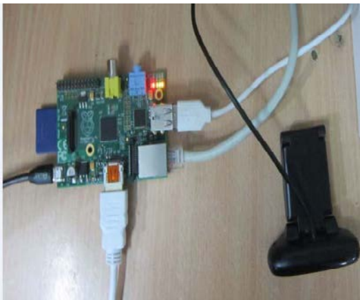
Fig 4: Connection Of USB Camera With Raspberry Pi
