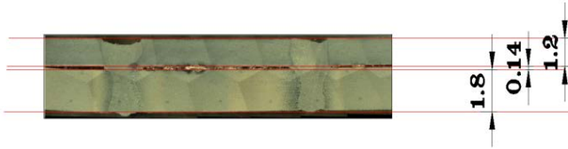
Fig. 9 Cross section of welding specimen
