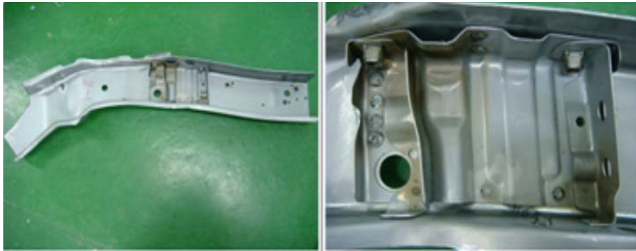
Fig. 10 Side member welded by laser
