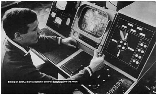
Fig. 2. Lunokhod control room, where from operators monitor and control the movements and operations of the vehicles with the help of visual feed-back [1]
