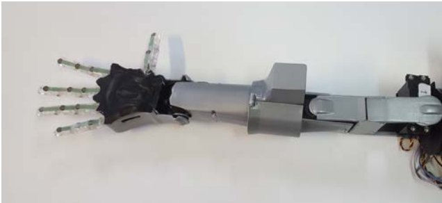
Fig. 5. Remotely operated robotic arm with pressure sensors on the fingers
