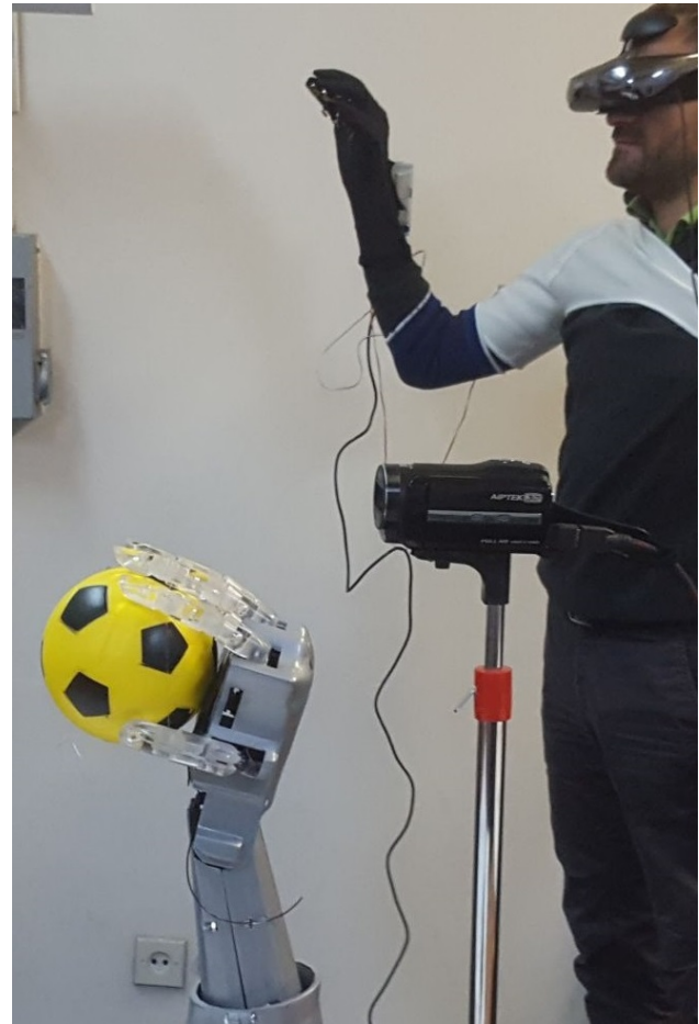
Fig. 9. Testing functioning robotic arm equipped with visual and haptic feedback channels
