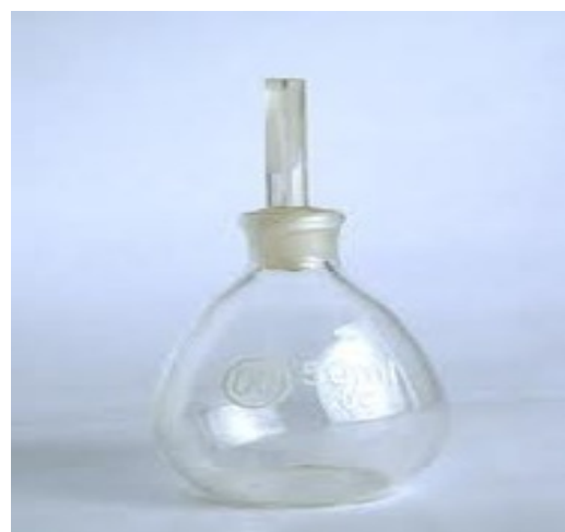
Fig 2- Relative density bottle for measurement of density
