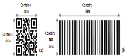
Fig. 1. Dimension for storing data in (a) 2D and (b) 1D codes.
