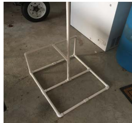
Fig. 4 Construction of PVC stand for small-scale model
