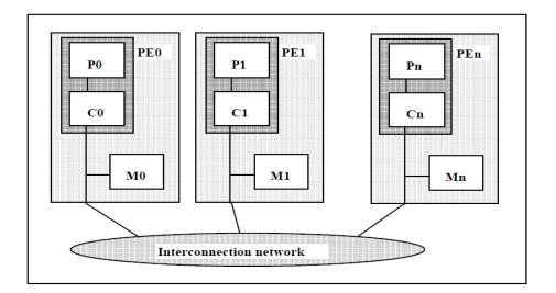
2. Cache-Only Memory Architecture (**COMA**) machines: In COMA machines every memory block works as a cache memory. Based on the applied cache coherence scheme data dynamically and continuously migrate to the local caches of those processors where the data are most needed.
