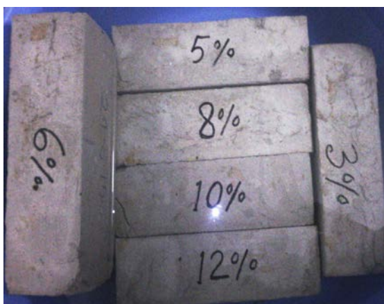
Figure-4: Submersion test of Compressed Stabilized Dredged Bricks Compressive strength:
