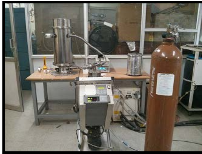
Fig. 4. Helium liquefaction setup using GM cryocooler
