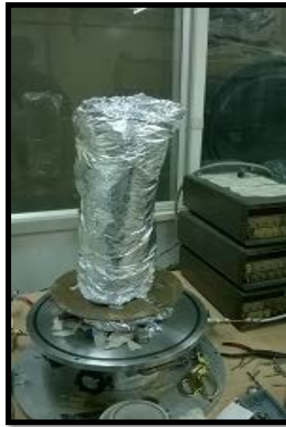
Fig. 3. Multilayer insulation applied to second stage and collection vessel
