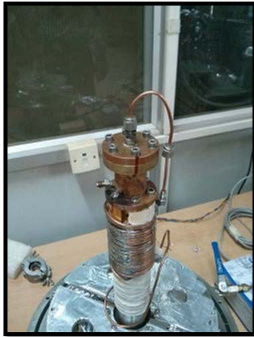
Fig. 2. GM cryocooler with heat exchanger and collection vessel mounted on second stage
