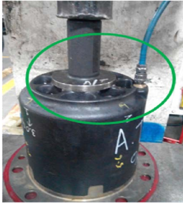
Air leak test 1.5 – 2 bar pressure
